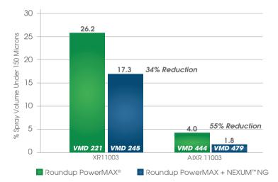
Volume median diameter (VMD) is the point where half the volume of spray is droplets larger than the VMD and half the volume is smaller. Low-Speed Wind Tunnel @ 43.5 psi - 2015
